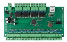
Door Control: Readers: 8 Exit Button: 4 Door Sensor Interface: 4 Relay: 4
