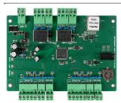
Door Control: 2 Readers: 4 Fxit Button: 2 Door Sensor Interface: 2 Relay: 2
