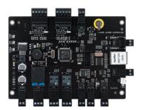
Door Control: 1 Readers: 2 Exit Button: 1 Door Sensor Interface: 1 Relay: 1
