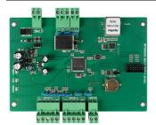
Door Control: 1 Readers: 2 Fxit Button: 1 Door Sensor Interface: 1 Relay: 1
